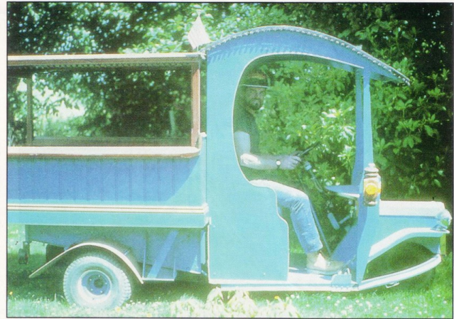
One of his first wooden vehicles, this Model T Depot Hack runs on a 2-cylinder gas engine and features redwood wainscoting.
