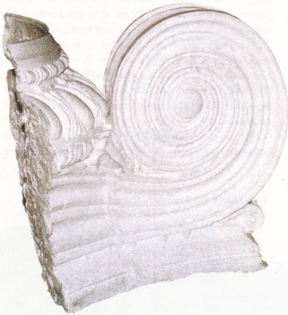
This plaster cornice was made in the Millwork's molding department.
